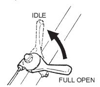
Figure 11. Throttle Lever (Idle)
